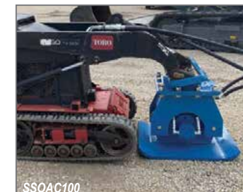
SSOAC100 24" wide tamper base plate, suitable for compact utility loaders.
